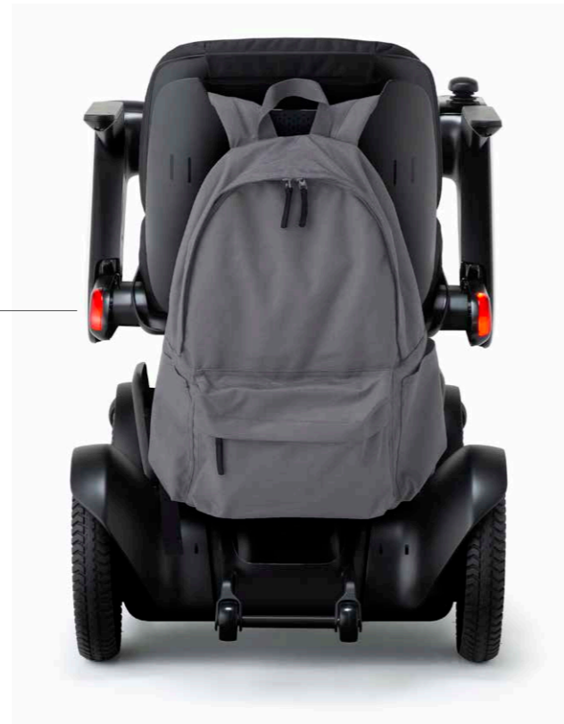
The tail light is clearly visible even with a bag hung over the back support, keeping you safe on the road at night.
